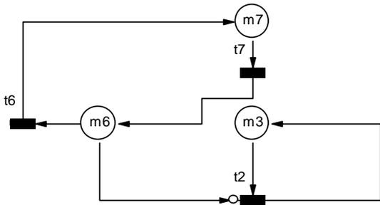
**Fig. 10. Kanban cell of Fig. 9 with idle subnet suppressed and similar to the abstract PN framework for logic tables in Fig. 6**
