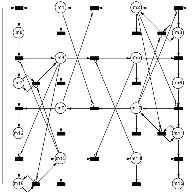
**Fig. 31. Alternate bit protocol model after Couvreur (1994, Fig. 7)**
