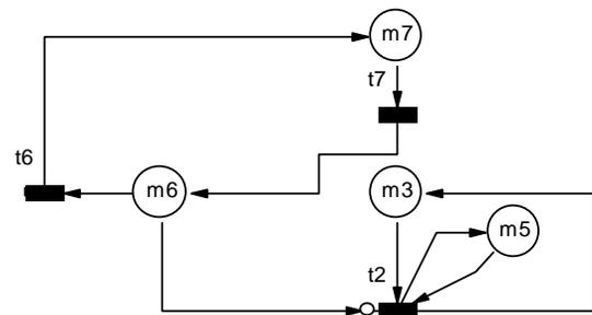
**Fig. 9. Reduced Kanban cell from Fig. 8**
