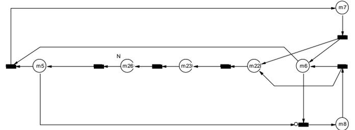
**Fig. 16. Reduced GSPN model from Fig. 15**
