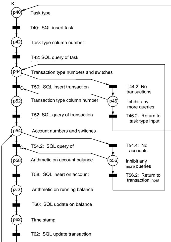
Fig. 2. PN for two logic tables (two dimensions)
