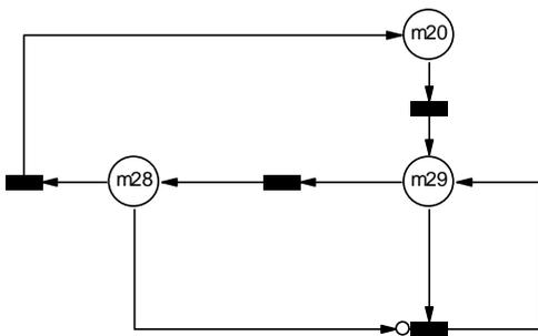
**Fig. 14. Reduced GSPN model from Fig. 13 and identical to the abstract PN framework for logic tables in Fig. 6**
