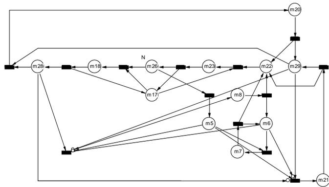
**Fig. 13. Reduced GSPN model from Fig. 12**
