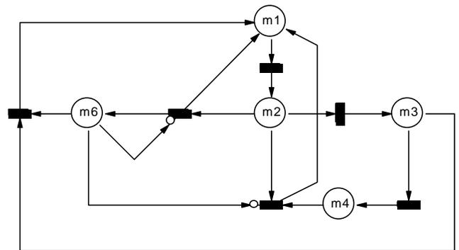
**Fig. 28. Redrawn GSPN model from Fig. 27**
