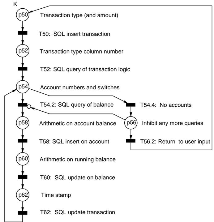
Fig 1. PN engine for one logic table
