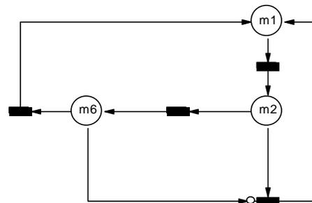
**Fig. 29. Reduced GSPN model from Fig. 28 and similar to the abstract PN framework for logic tables in Fig. 6**
